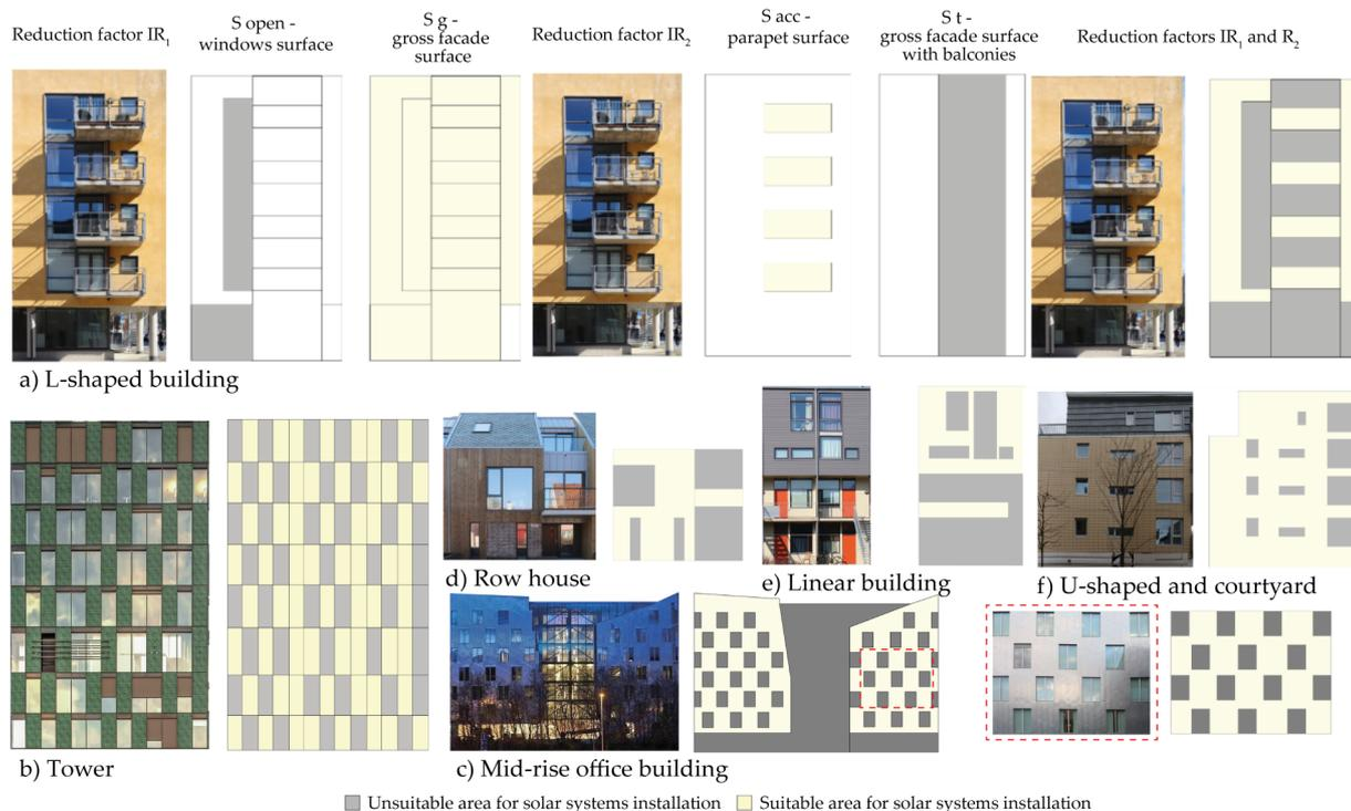
Graphical calculation in AutoCAD of the reduction factors IR<sub>1</sub> and IR<sub>2</sub> for L-shaped building and summary of the calculation of factors for all building morphologies
