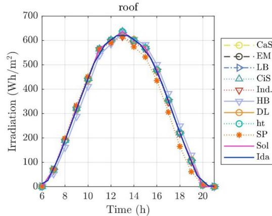
Figure 15 Hourly irradiation received on the roof in February
