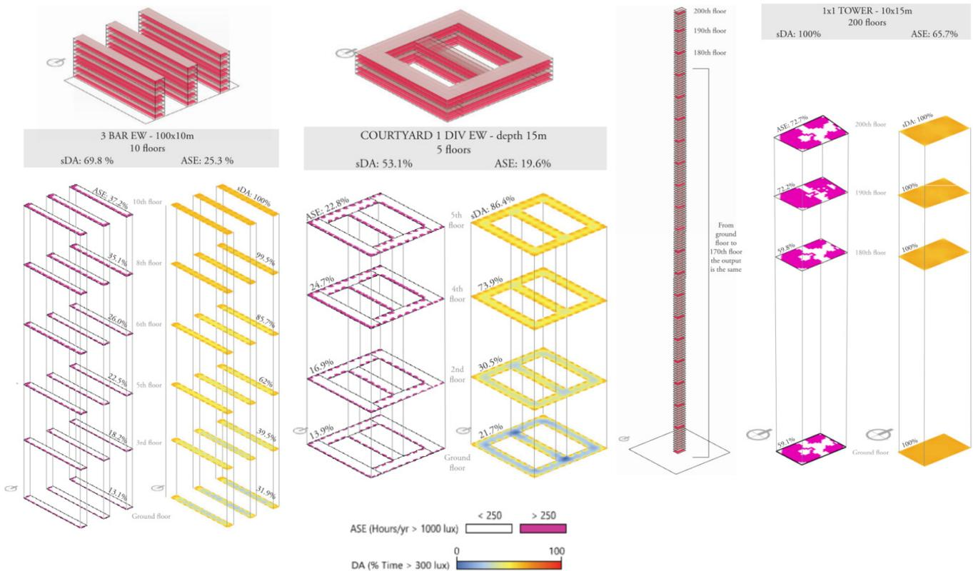
Example of one type of simulation using DIVA (Solemma): Spatial Daylight Autonomy
