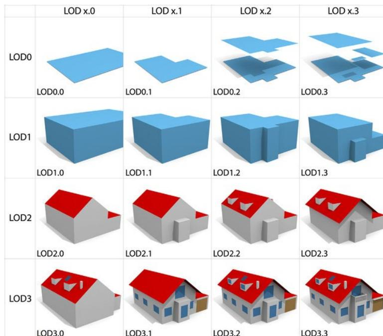
**Figure 4: different Levels of Detail illustrated. Illustration under CC agreement (Biljecki et al., 2016)**
