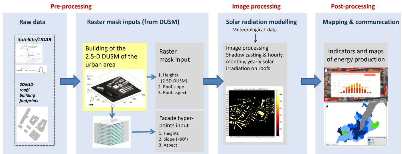
Workflow of the whole process of solar modelling on roofs and facades. Source: <https://doi.org/10.3390/app10155361>
