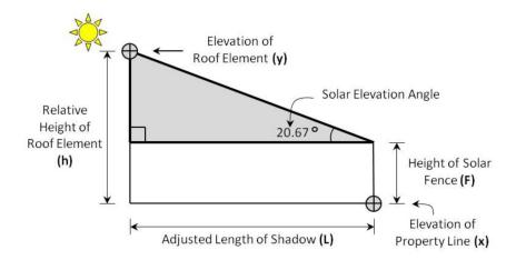
Figure 17: Section along Shadow Length at 10 AM
